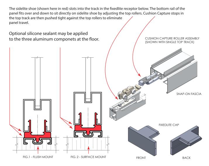
5/16" high fixedlite receptor must be installed on a firm surface using construction adhesive.
