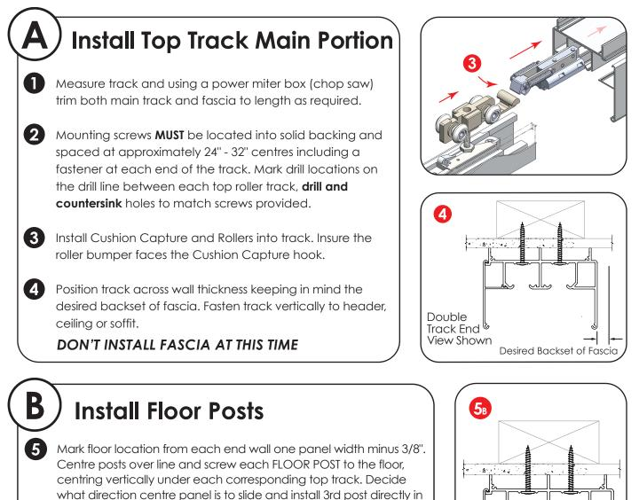
**IMPORTANT NOTE:** Sliding Panel Rail End Cap should never come in contact with the floor post. (See "PANEL ADJUSTMENT")
