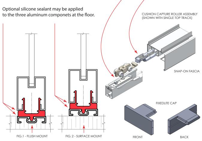
5/16" high fixedlite receptor must be installed on a firm surface using construction adhesive.
