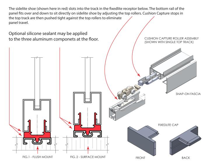
5/16" high fixedlite receptor must be installed on a firm surface using construction adhesive.
