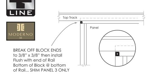
BREAK OFF at notches to yield 2 Collector blocks (discard middle section)
