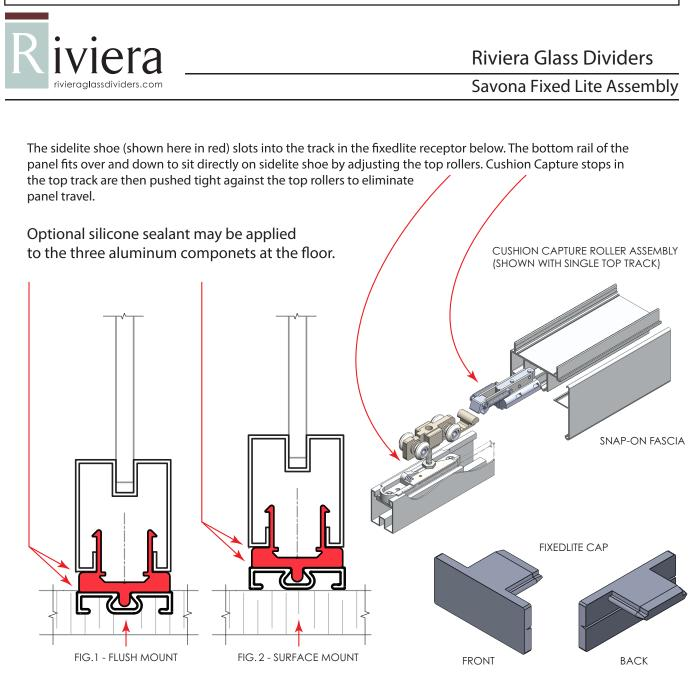
5/16" high fixedlite receptor must be installed on a firm surface using construction adhesive.
